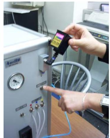
Adjust the ink volume. Close the cover of the filling chamber firmly and push to the start/stop button, it will start vacuuming and when reached to the correct vacuum level , automatically filling will start filling and stop after filling completed. Take out the cartridge from the Filling Chamber using the suction cup , do the priming operation , now it is ready to print test.
