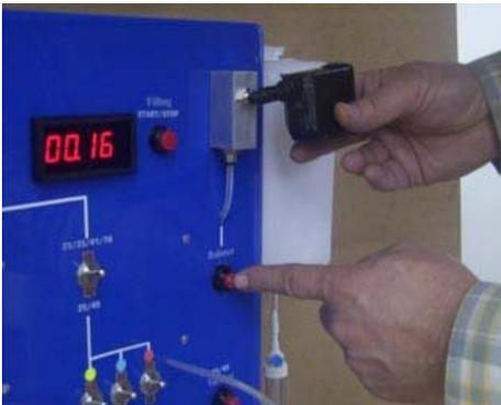
Swing suction cup to horizontal position. Hold cartridge with circuitry facing upwards, Apply low vacuum in one second pulses to remove ink channel bubbles, if present.
