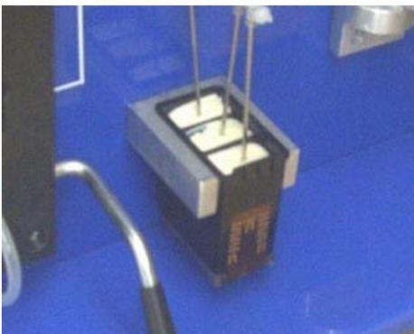
**Place the cartridge into the filling station**
