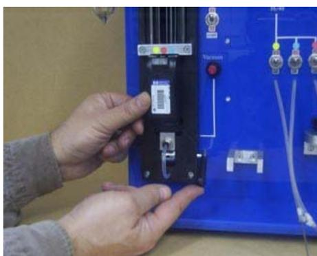
**Lift the handle up and squeeze the cartridge**
