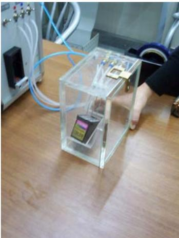
Place the cartridge inside of the filling chamber.
