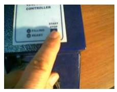
Push the Start / Stop Button to start the filling operation
