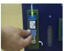
Place the cartridge in to the filling station.
