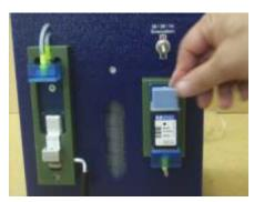
For start up the cartridge, replace the cartridge into evacuation station and do evacuation 3-4 seconds, then remove cartridge and test it.
