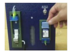
Place the cartridge in to the evacuation station if necessary
