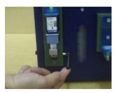
Then remove the cartridge using the handle
