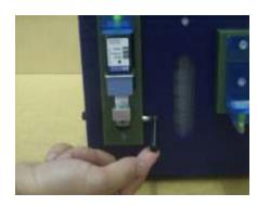
Secure the cartridge by pushing the handle up.
