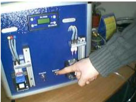
After filling has completed flip down the Evacuation station 2-3 seconds for priming the cartridge, Bring the top position the needles and take out the cartridge from station and test it.
