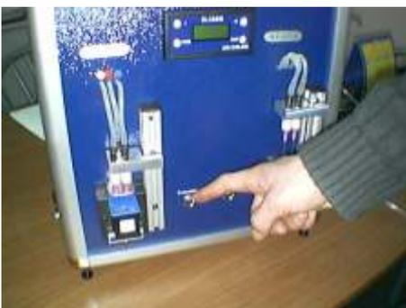
Flip down the switch to start evacuation to empty the cartridge first, it will be empty in 20-30 seconds.
