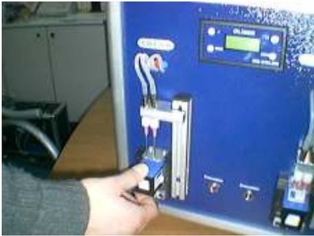
Take out the top label of cartridge and place the color cartridge in to the evacuation/filling station .
