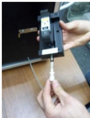
Insert the cartridge into the cradle , connect the filling tube. Place the cradle on the machine.
