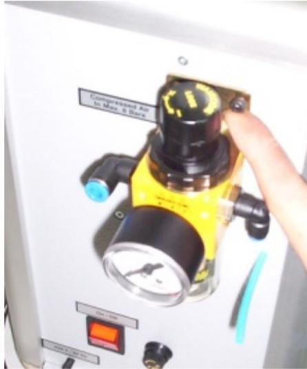
Pressure Regulator will be shipped you separately , so first you will install it the place of it as shown above left side of the machine. Two screws are provided for the installation of pressure regulator , screw them together with the pressure regulator and fix it on the left side of the machine, connect the inlet tube to the pressure regulator and connect compressed air tube (6mm) to the pressure regulator as shown shown right.
