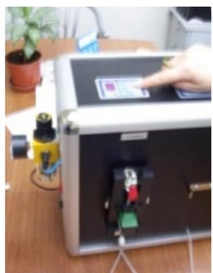
Insert the cartridge into the cradle , connect the cleaning&evacuation tube. Place the cradle on the machine.
