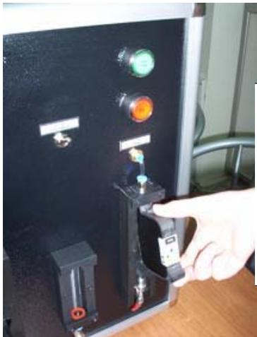
Then insert the cartridge to the filling station, and secure the cartridge flipping up the red handle
