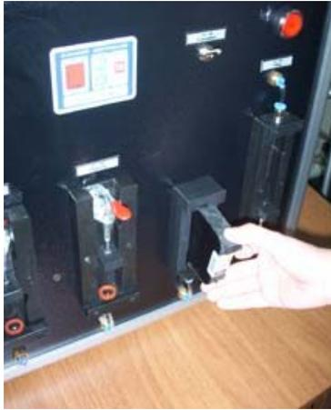
Place the cartridge in to the 15/45 evacuation station after Flip down the Evacuation button to start emptying the cartridge.
