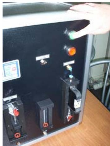
Push Start / Stop button. It will do 20 seconds vacuum and at the same time syringe will be filled by ink , then syringe movement will start to fill the cartridge in 20-30 seconds.
