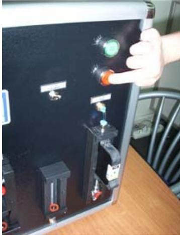
When the cartridge filled (piston movement is stopped) push to the balance button 3-5 seconds and take out the cartridge for print test.
